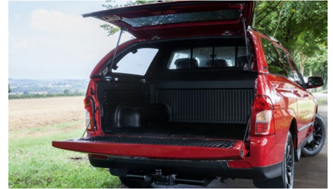
Moulded Hard Top – full hard top with brake lights, headed rear window, sliding front glass, LED interior light, central locking, pop out opening windows & roof bars
