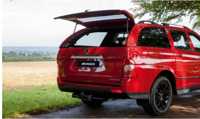
Moulded Hard Top – full hard top with brake lights, headed rear window, sliding front glass, LED interior light, central locking, pop out opening windows & roof bars
