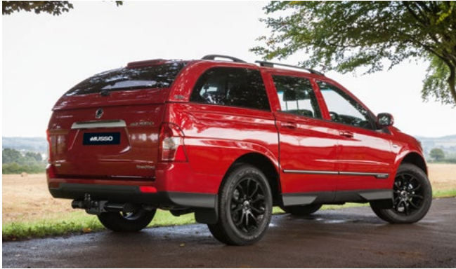
Moulded Hard Top – full hard top with brake lights, headed rear window, sliding front glass, LED interior light, central locking, pop out opening windows & roof bars
